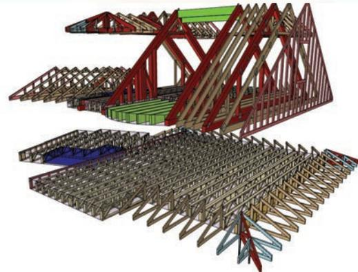
*“With trusses, building the roof is more like putting the pieces of a puzzle together, because the engineering has already been done off site by the component manufacturer,” said George Aiken. “You are piecing together a roof system that’s already been configured; you are not framing the roof from scratch each time.”*
